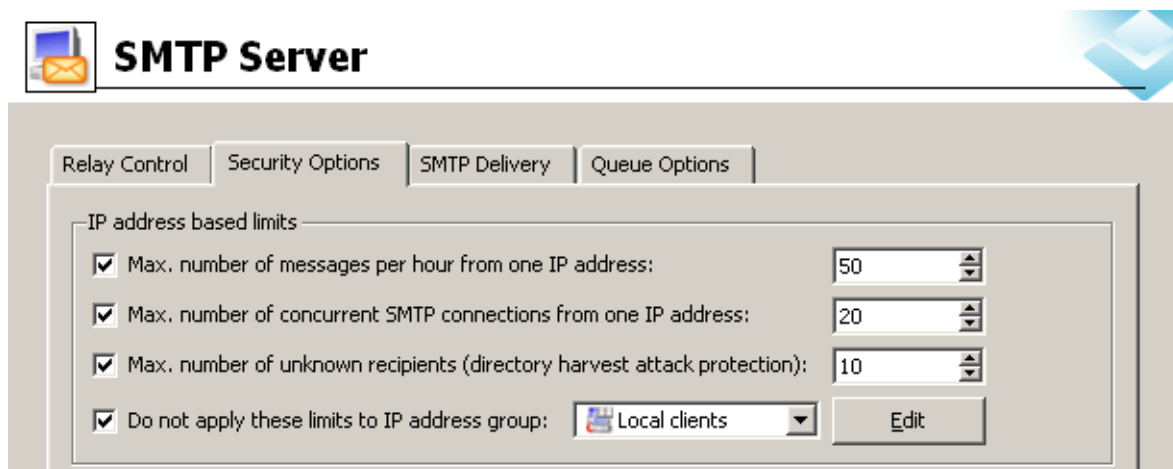
Figure 12.2 Security Options — IP address based limits
