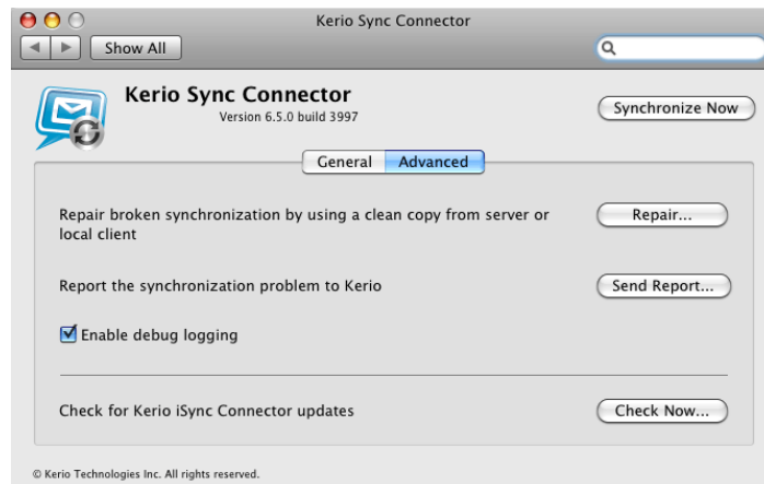
Figure 40.2 Log settings in Kerio Sync Connector
